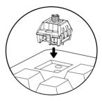
STEP 4: Inserting a new switch.
