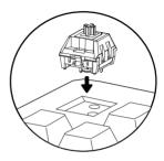
STEP 4: Inserting a new switch.
