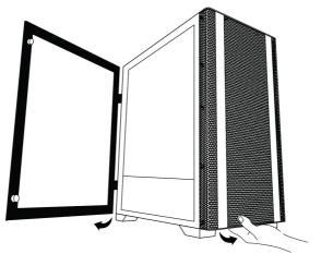
Open the front cover by pulling outwards from the bottom of the panel.
