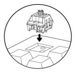
STEP 4: Inserting a new switch.
