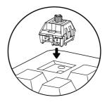
STEP 4: Inserting a new switch.
