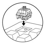
STEP 4: Inserting a new switch.
