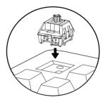
STEP 4: Inserting a new switch.
